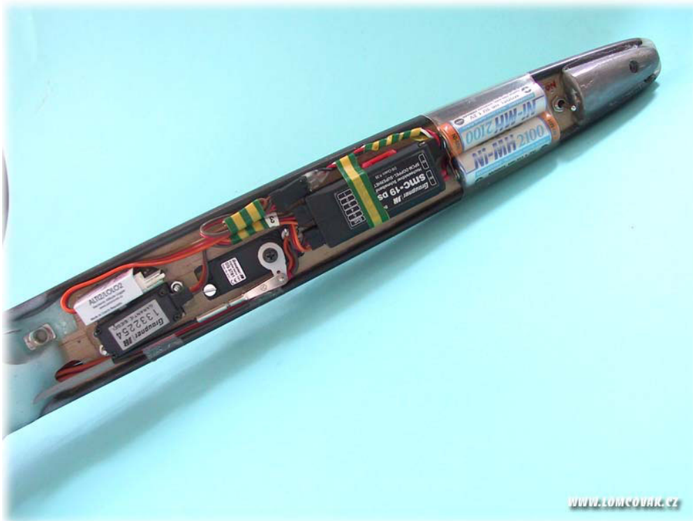
A2 installation in F3B Caracho 3.1 Plus
